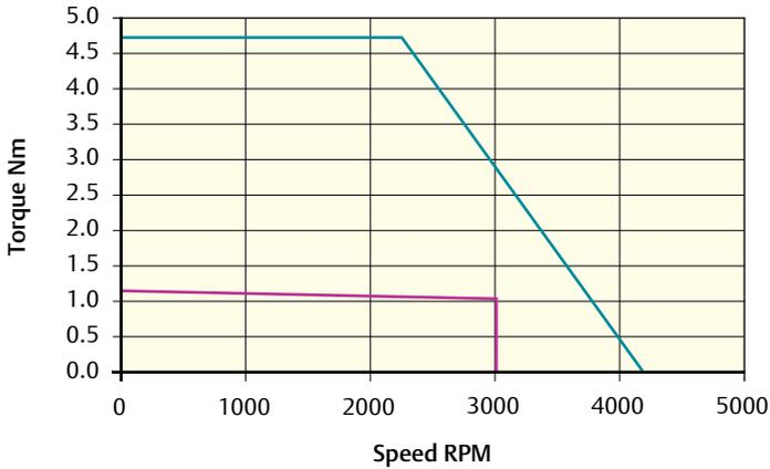
Peak torque (Nm) = 4.72    Stall torque (Nm) = 1.18    Rated torque (Nm) = 1.05
