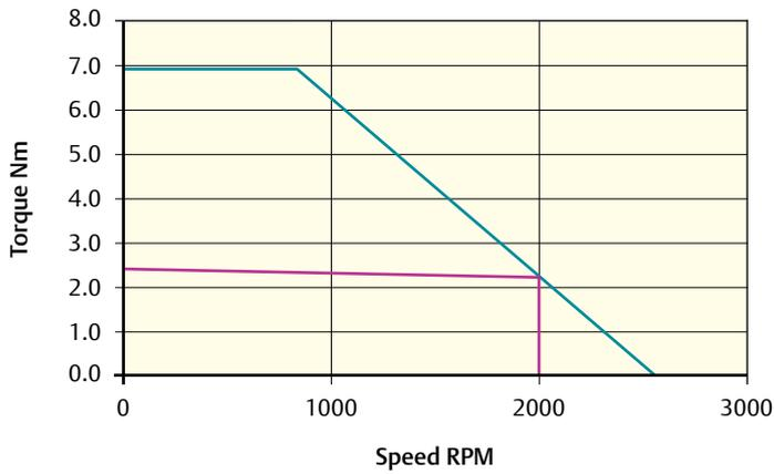
Peak torque (Nm) = 6.9    Stall torque (Nm) = 2.3    Rated torque (Nm) = 2.2
