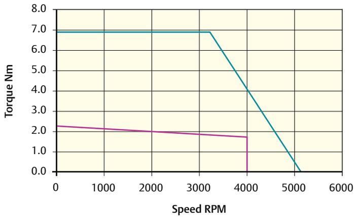
Peak torque (Nm) = 6.9    Stall torque (Nm) = 2.3    Rated torque (Nm) = 1.8
