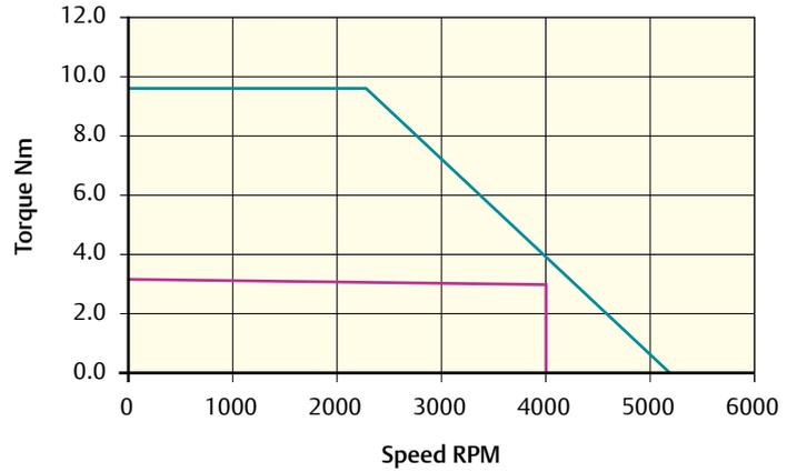
Peak torque (Nm) = 9.60 Stall torque (Nm) = 3.20 Rated torque (Nm) = 2.90
