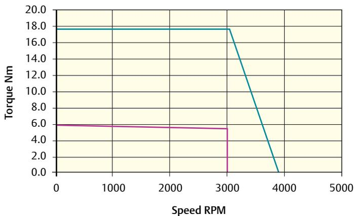
Peak torque (Nm) = 17.7    Stall torque (Nm) = 5.9    Rated torque (Nm) = 5.4
