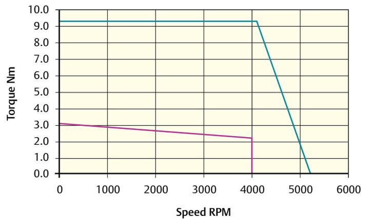
Peak torque (Nm) = 9.3    Stall torque (Nm) = 3.1    Rated torque (Nm) = 2.3
