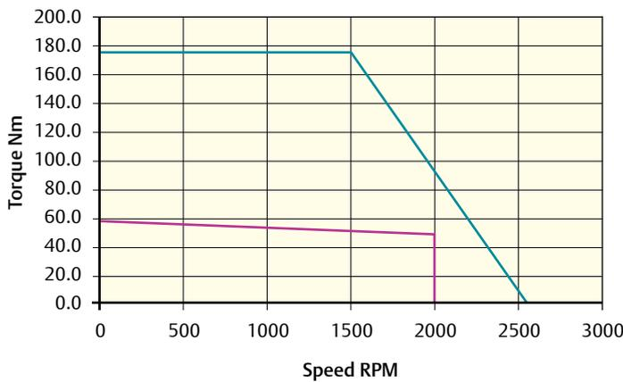
Peak torque (Nm) = 176.1   Stall torque (Nm) = 58.7   Rated torque (Nm) = 50.4
