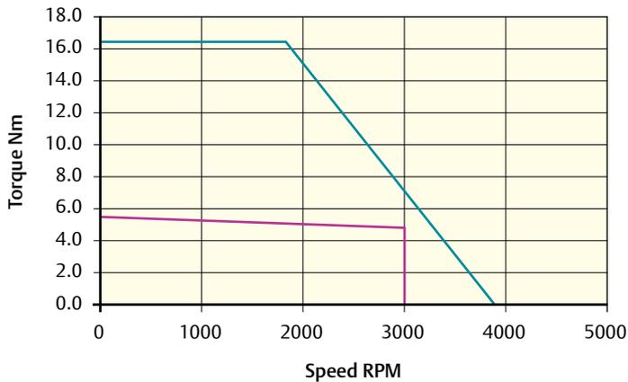
Peak torque (Nm) = 16.50 Stall torque (Nm) = 5.50 Rated torque (Nm) = 4.85
