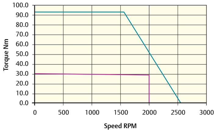
Peak torque (Nm) = 93.3    Stall torque (Nm) = 31.1    Rated torque (Nm) = 28.4
