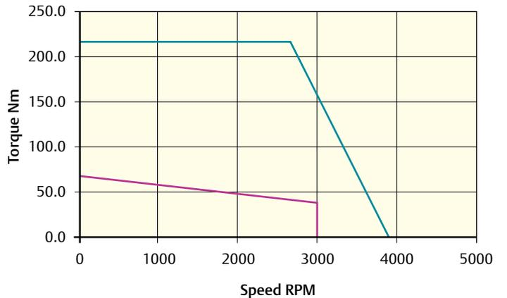
Peak torque (Nm) = 219.6 Stall torque (Nm) = 73.2 Rated torque (Nm) = 36.8
