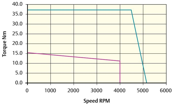
Peak torque (Nm) = 37.20 Stall torque (Nm) = 15.2 Rated torque (Nm) = 12.0
