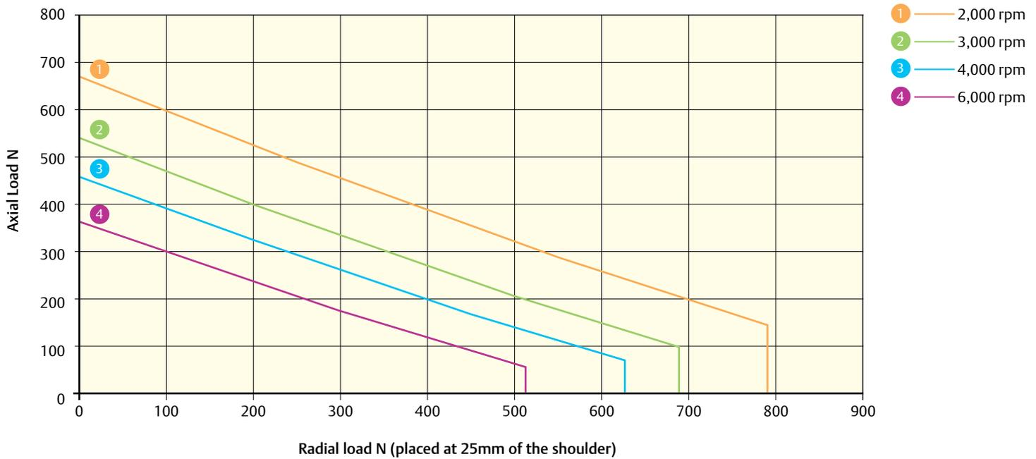
089UD  $L_{10(h)}$  Bearing life for 20,000 hours (reliability 90%, load factor of 1). Do not exceed a maximum axial load of 1000 N
