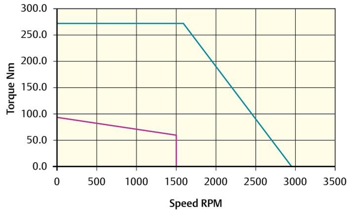
Peak torque (Nm) = 276.0 Stall torque (Nm) = 92.0 Rated torque (Nm) = 62.0
