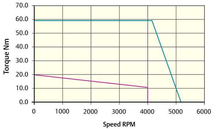
Peak torque (Nm) = 59.4    Stall torque (Nm) = 19.8    Rated torque (Nm) = 10.7
