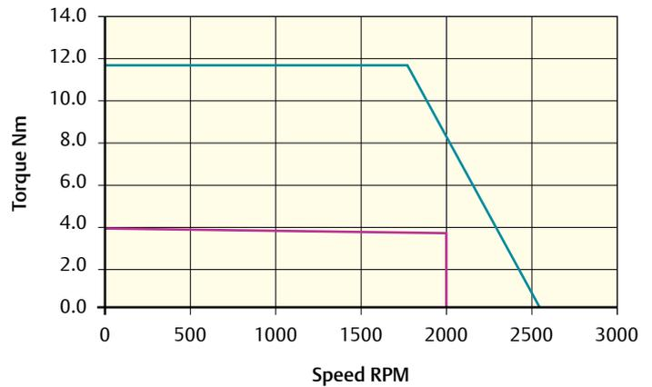
Peak torque (Nm) = 11.7    Stall torque (Nm) = 3.9    Rated torque (Nm) = 3.8
