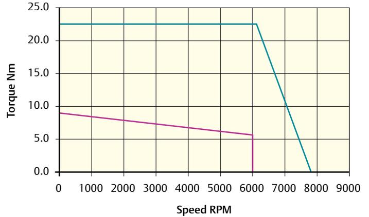
Peak torque (Nm) = 22.50 Stall torque (Nm) = 9.0 Rated torque (Nm) = 5.8
