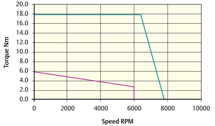
Peak torque (Nm) = 17.7    Stall torque (Nm) = 5.9    Rated torque (Nm) = 2.8
