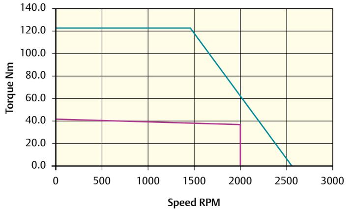
Peak torque (Nm) = 123.3    Stall torque (Nm) = 41.1    Rated torque (Nm) = 36.9
