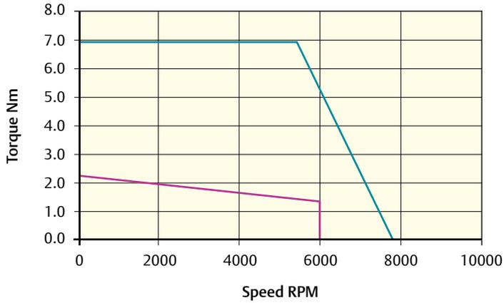
Peak torque (Nm) = 6.9    Stall torque (Nm) = 2.3    Rated torque (Nm) = 1.3
