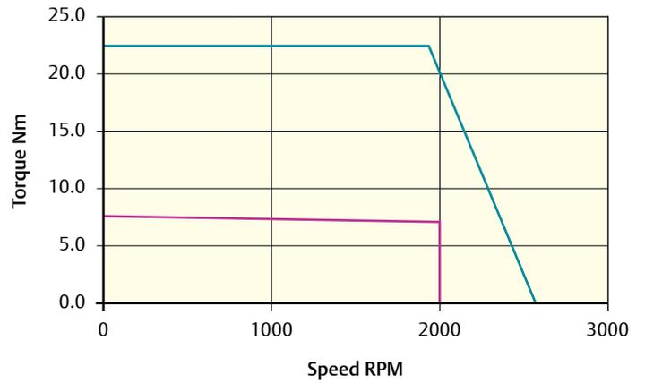
Peak torque (Nm) = 22.5    Stall torque (Nm) = 7.5    Rated torque (Nm) = 6.9
