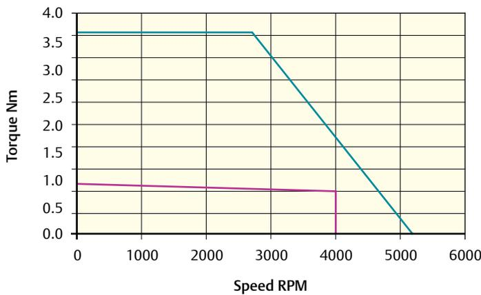
Peak torque (Nm) = 3.6    Stall torque (Nm) = 1.2    Rated torque (Nm) = 1.0
