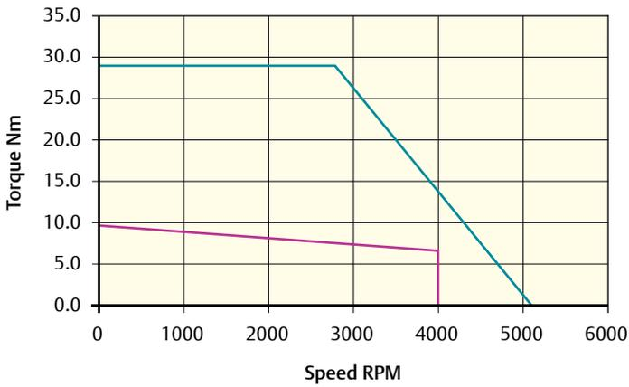
Peak torque (Nm) = 28.8    Stall torque (Nm) = 9.6    Rated torque (Nm) = 7.0
