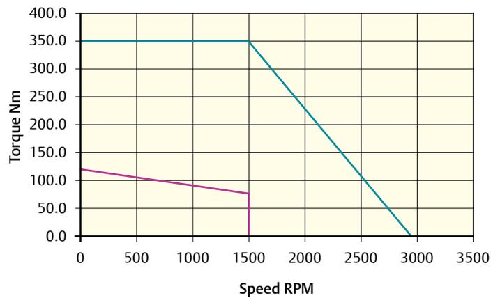
Peak torque (Nm) = 348.0 Stall torque (Nm) = 116.0 Rated torque (Nm) = 70.0
