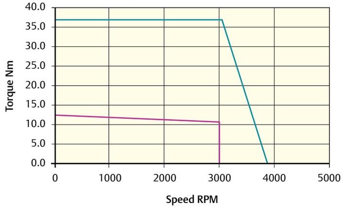
Peak torque (Nm) = 37.4    Stall torque (Nm) = 12.4    Rated torque (Nm) = 10.4
