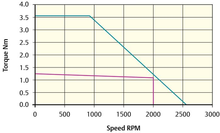
Peak torque (Nm) = 3.6    Stall torque (Nm) = 1.2    Rated torque (Nm) = 1.1
