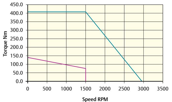
Peak torque (Nm) = 408.0 Stall torque (Nm) = 136.0 Rated torque (Nm) = 77.0
