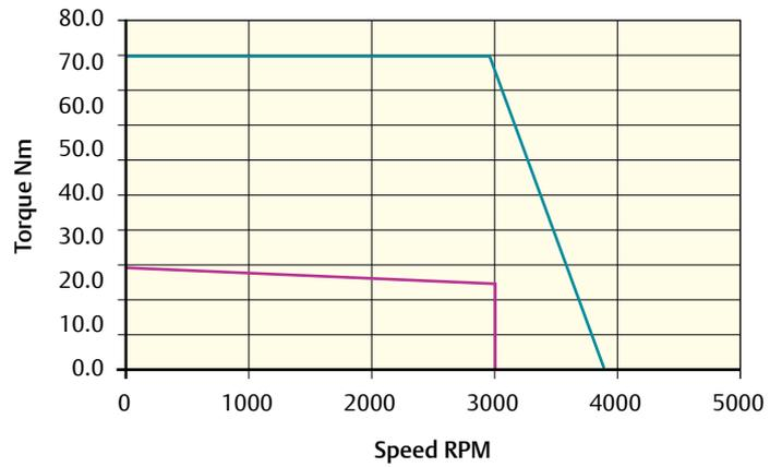
Peak torque (Nm) = 70.20 Stall torque (Nm) = 29.5 Rated torque (Nm) = 25.0
