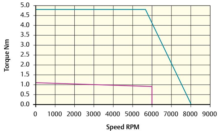
Peak torque (Nm) = 4.72    Stall torque (Nm) = 1.18    Rated torque (Nm) = 0.90
