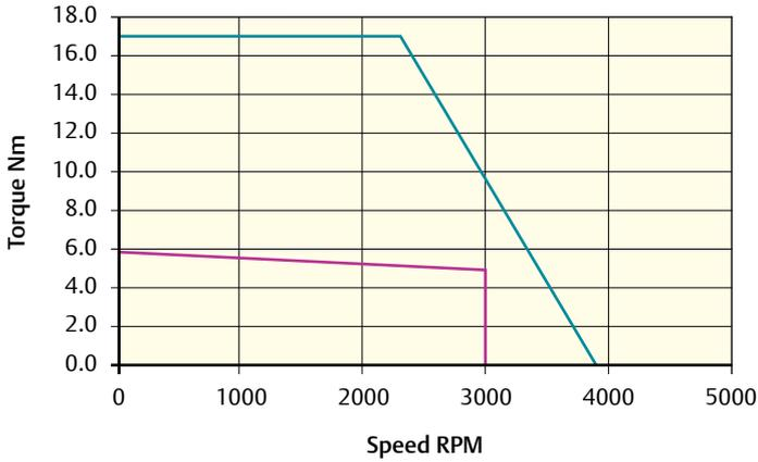
Peak torque (Nm) = 17.1    Stall torque (Nm) = 5.7    Rated torque (Nm) = 4.9
