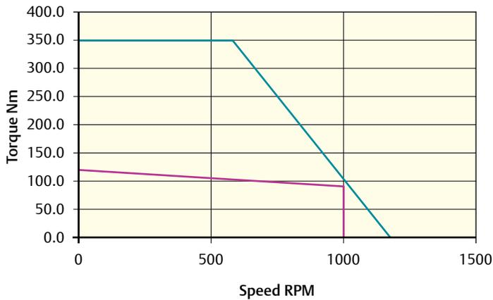
Peak torque (Nm) = 348.0 Stall torque (Nm) = 116.0 Rated torque (Nm) = 92.0
