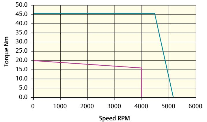
Peak torque (Nm) = 45.90 Stall torque (Nm) = 20.1 Rated torque (Nm) = 16.1
