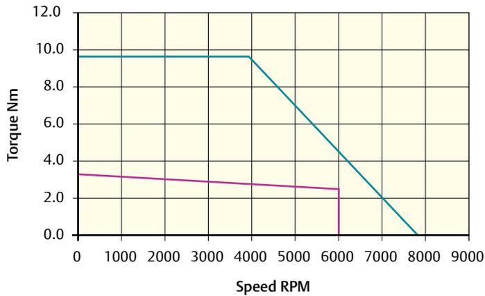
Peak torque (Nm) = 9.60    Stall torque (Nm) = 3.20    Rated torque (Nm) = 2.65
