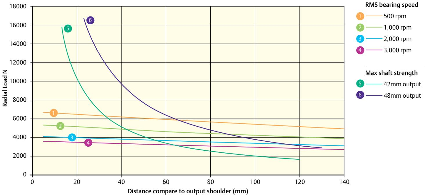
250U2 L<sub>10(h)</sub> Bearing life for 20,000 hours (reliability 90%, load factor of 1)
