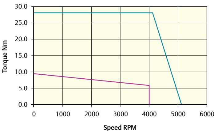
Peak torque (Nm) = 28.2    Stall torque (Nm) = 9.4    Rated torque (Nm) = 6.3
