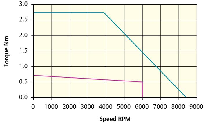
Peak torque (Nm) = 2.8    Stall torque (Nm) = 0.7    Rated torque (Nm) = 0.5
