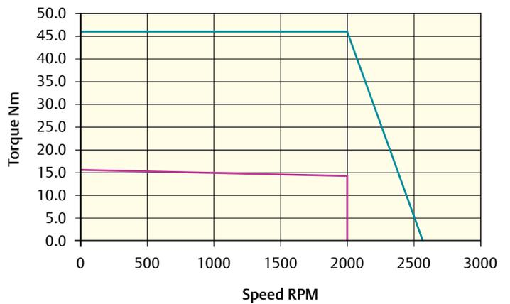
Peak torque (Nm) = 45.9    Stall torque (Nm) = 15.3    Rated torque (Nm) = 14.0
