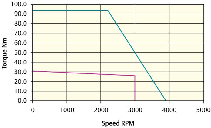
Peak torque (Nm) = 93.3 Stall torque (Nm) = 31.1 Rated torque (Nm) = 25.0
