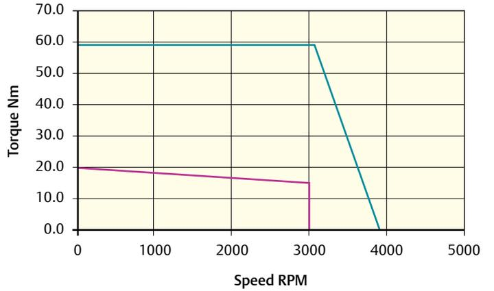
Peak torque (Nm) = 59.4    Stall torque (Nm) = 19.8    Rated torque (Nm) = 15.8
