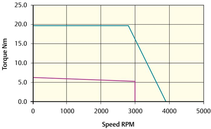
Peak torque (Nm) = 19.8    Stall torque (Nm) = 6.6    Rated torque (Nm) = 5.5
