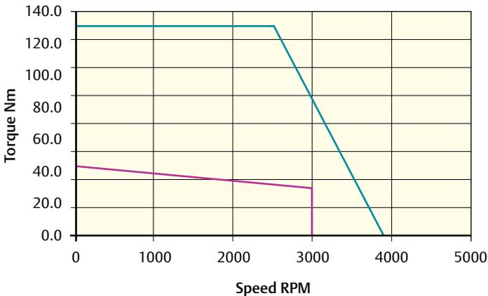
Peak torque (Nm) = 151.6 Stall torque (Nm) = 50.6 Rated torque (Nm) = 34.0
