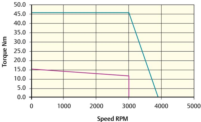
Peak torque (Nm) = 45.9    Stall torque (Nm) = 15.3    Rated torque (Nm) = 12.2
