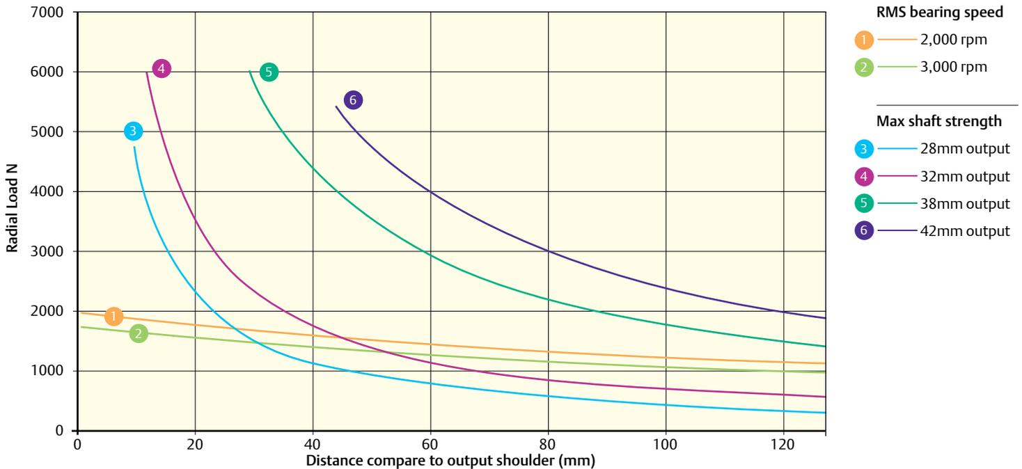
190U2 L<sub>10(h)</sub> Bearing life for 20,000 hours (reliability 90%, load factor of 1)
