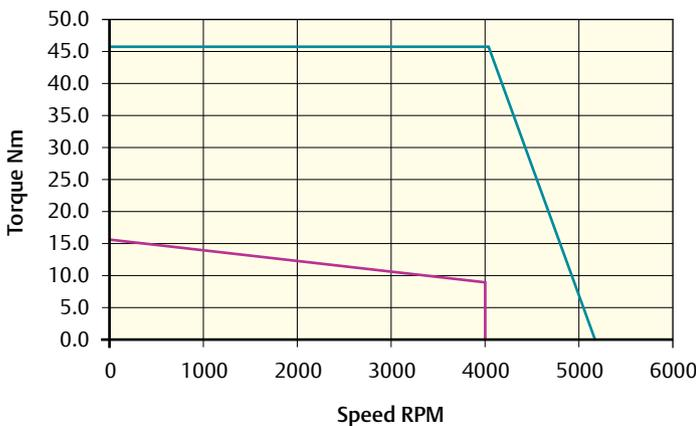
Peak torque (Nm) = 45.9    Stall torque (Nm) = 15.3    Rated torque (Nm) = 8.9
