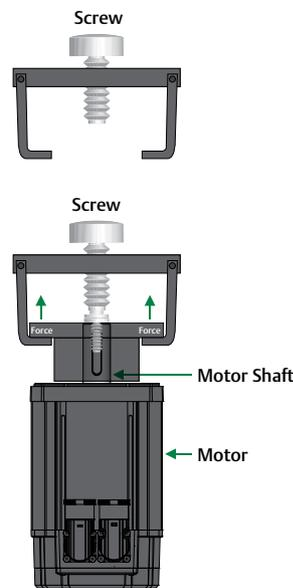
To remove pulleys a two or three legged gear puller must be used.
