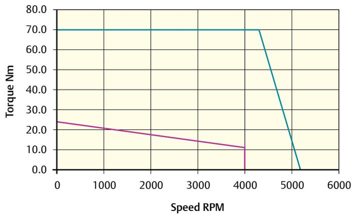
Peak torque (Nm) = 70.2    Stall torque (Nm) = 23.4    Rated torque (Nm) = 12.2
