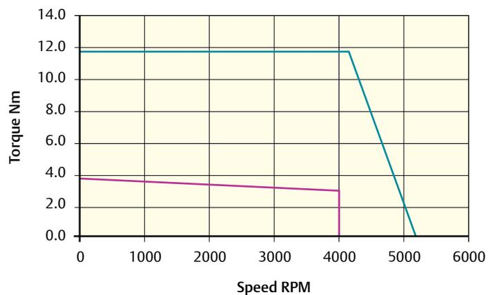
Peak torque (Nm) = 11.7    Stall torque (Nm) = 3.9    Rated torque (Nm) = 2.9
