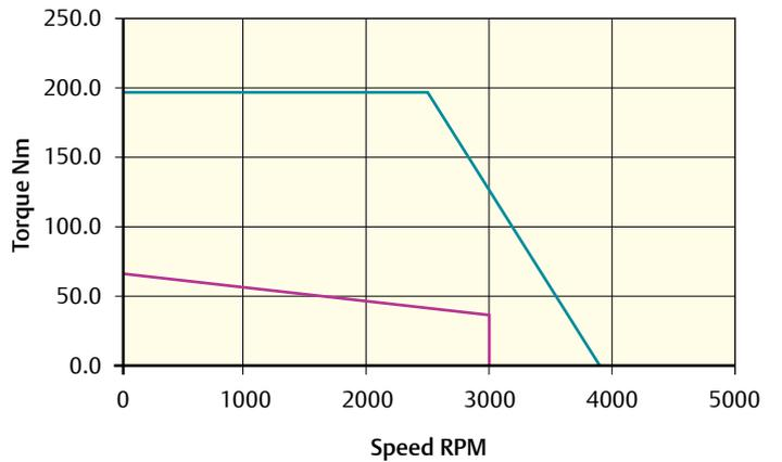
Peak torque (Nm) = 198.0 Stall torque (Nm) = 66.0 Rated torque (Nm) = 36.0
