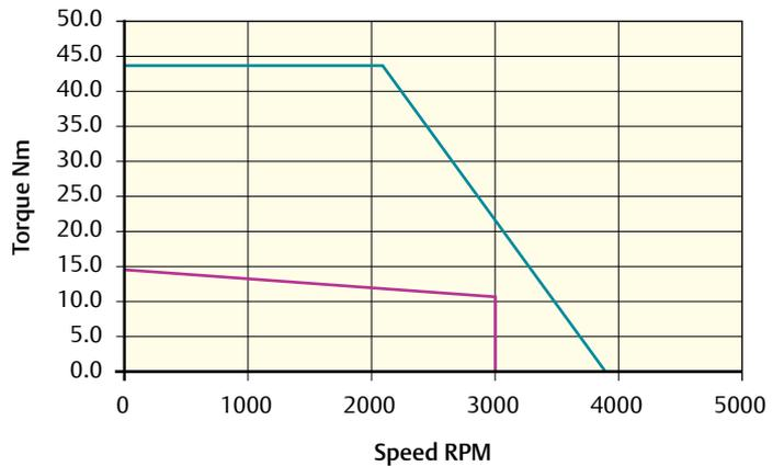
Peak torque (Nm) = 43.80 Stall torque (Nm) = 14.60 Rated torque (Nm) = 10.50
