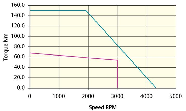
Peak torque (Nm) = 151.6 Stall torque (Nm) = 68.0 Rated torque (Nm) = 55.0
