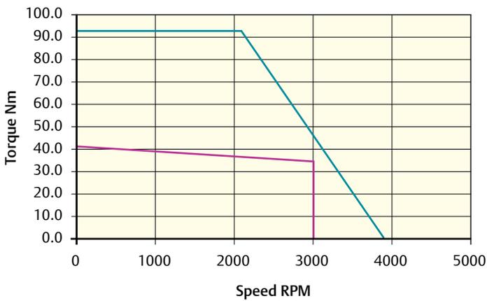
Peak torque (Nm) = 93.30 Stall torque (Nm) = 41.0 Rated torque (Nm) = 35.5
