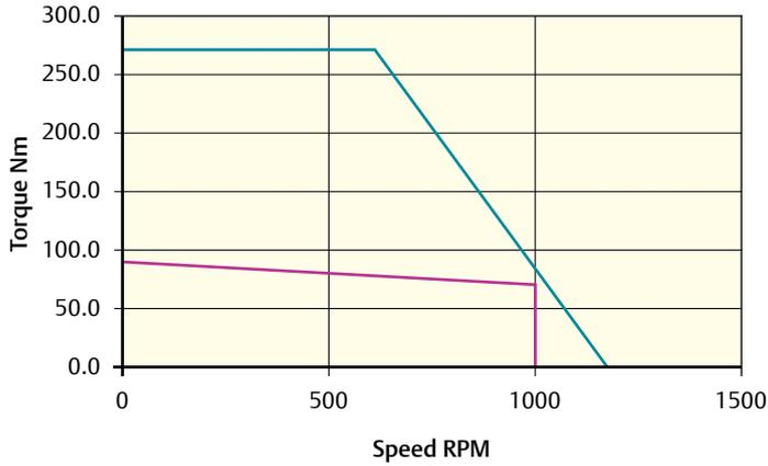
Peak torque (Nm) = 276.0 Stall torque (Nm) = 92.0 Rated torque (Nm) = 75.0
