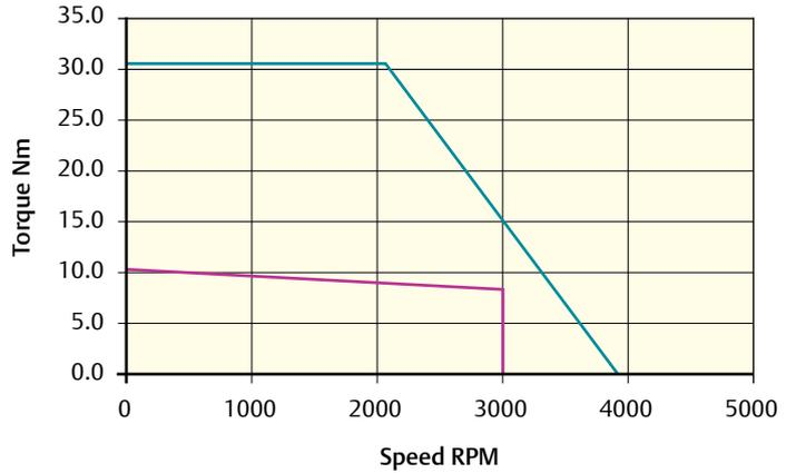
Peak torque (Nm) = 30.60 Stall torque (Nm) = 10.20 Rated torque (Nm) = 7.70
