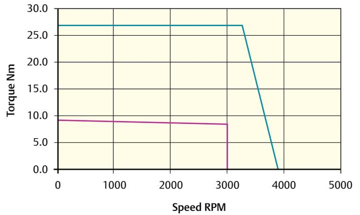
Peak torque (Nm) = 27.0    Stall torque (Nm) = 9.0    Rated torque (Nm) = 8.1
