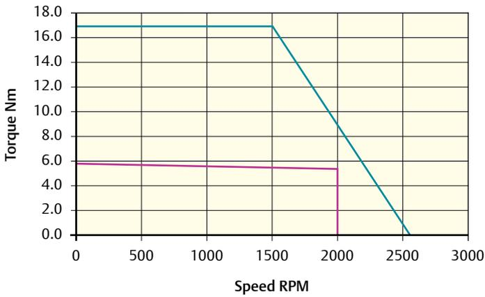
Peak torque (Nm) = 17.1    Stall torque (Nm) = 5.7    Rated torque (Nm) = 5.3
