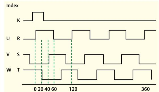
Where  $N$  = number of poles. For example a 6 pole motor the encoder commutation tracks will output 3 pulses per channel per revolution and for an 8 pole motor the encoder commutation tracks will give 4 pulses per channel per revolution.
