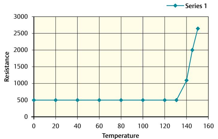
The installer must connect the motor thermistor to the drive to cause motor power shutdown in the event of overheating. It is the installer's responsibility to ensure that this protection facility is properly connected and set at the drive.
