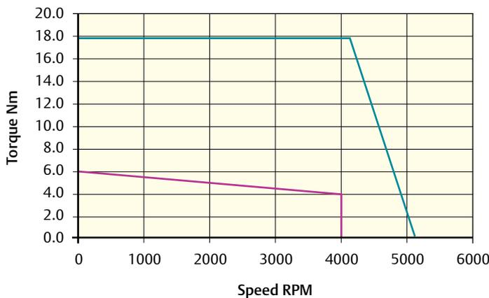
Peak torque (Nm) = 17.7    Stall torque (Nm) = 5.9    Rated torque (Nm) = 4.0
