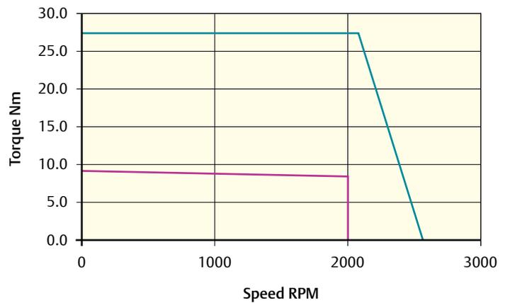
Peak torque (Nm) = 27.0    Stall torque (Nm) = 9.0    Rated torque (Nm) = 8.2
