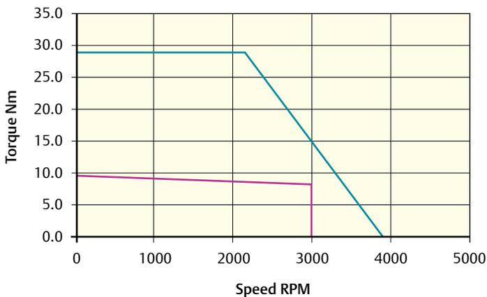
Peak torque (Nm) = 28.8   Stall torque (Nm) = 9.6   Rated torque (Nm) = 8.7
