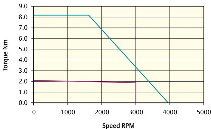
Peak torque (Nm) = 8.3    Stall torque (Nm) = 2.1    Rated torque (Nm) = 1.8
