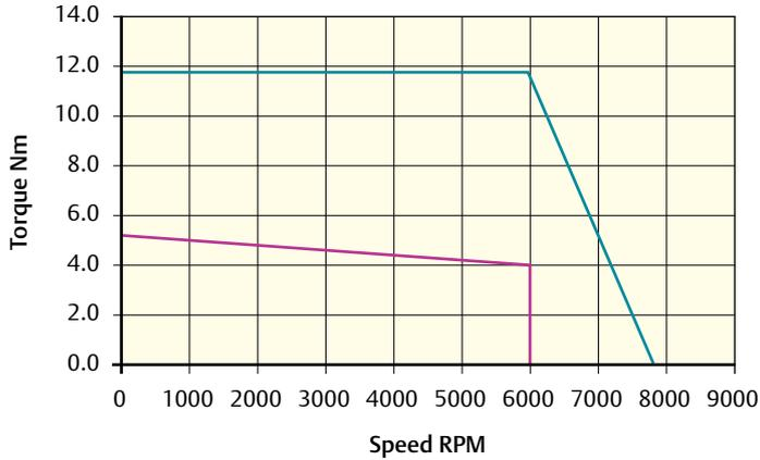
Peak torque (Nm) = 11.70 Stall torque (Nm) = 5.2 Rated torque (Nm) = 4.0
