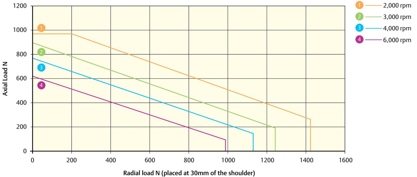
115U2  $L_{10(h)}$  Bearing life for 20,000 hours (reliability 90%, load factor of 1). Do not exceed a maximum axial load of 950 N
