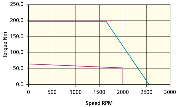
Peak torque (Nm) = 198.0   Stall torque (Nm) = 66.0   Rated torque (Nm) = 53.0
