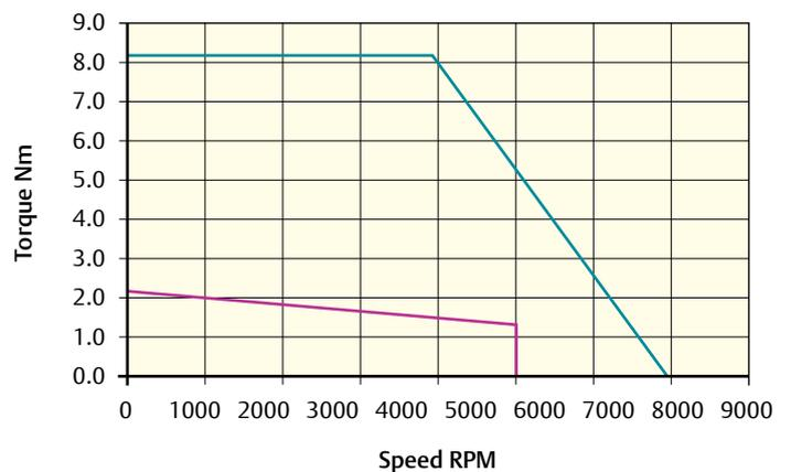
Peak torque (Nm) = 8.3    Stall torque (Nm) = 2.1    Rated torque (Nm) = 1.4
