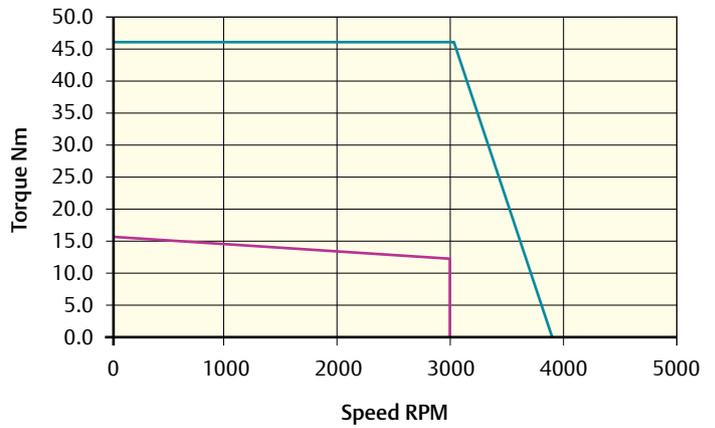
Peak torque (Nm) = 45.9    Stall torque (Nm) = 15.3    Rated torque (Nm) = 12.6
