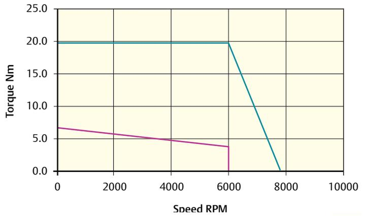
Peak torque (Nm) = 19.8    Stall torque (Nm) = 6.6    Rated torque (Nm) = 4.0
