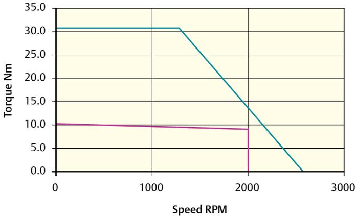
Peak torque (Nm) = 30.60 Stall torque (Nm) = 10.20 Rated torque (Nm) = 8.60
