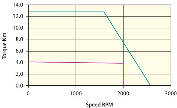
Peak torque (Nm) = 12.9    Stall torque (Nm) = 4.3    Rated torque (Nm) = 4.0
