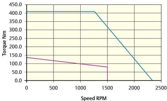
Peak torque (Nm) = 408.0 Stall torque (Nm) = 136.0 Rated torque (Nm) = 81.0
