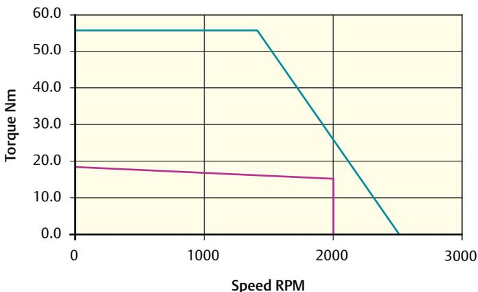
Peak torque (Nm) = 56.40 Stall torque (Nm) = 18.80 Rated torque (Nm) = 15.60
