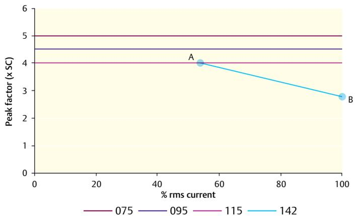
As shown above the 075 increases to 5 times, 095 increases to 4.5 times, the 115 increases to 4 times across the % rms current line and the 142 shows an increase to 4 times up until 57% dropping to 2.5 times at 100%.
