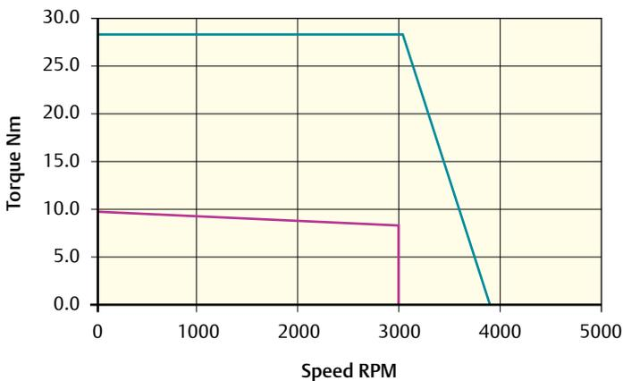
Peak torque (Nm) = 28.2    Stall torque (Nm) = 9.4    Rated torque (Nm) = 8.1
