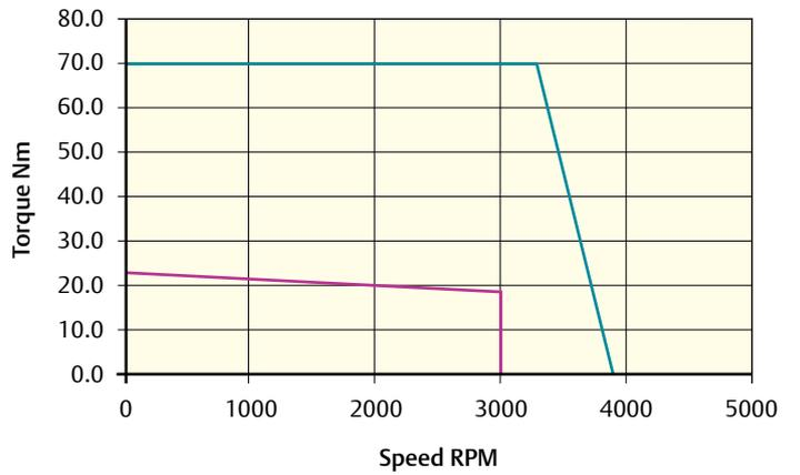
Peak torque (Nm) = 70.2    Stall torque (Nm) = 23.4    Rated torque (Nm) = 18.0
