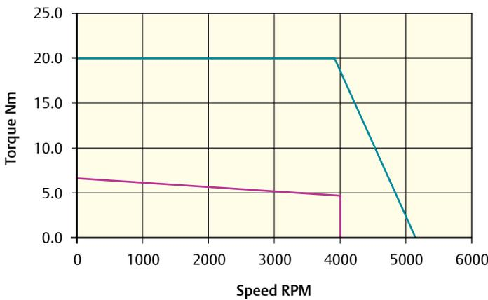
Peak torque (Nm) = 19.8    Stall torque (Nm) = 6.6    Rated torque (Nm) = 4.7
