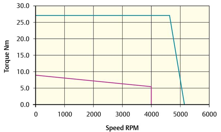
Peak torque (Nm) = 27.0    Stall torque (Nm) = 9.0    Rated torque (Nm) = 5.7
