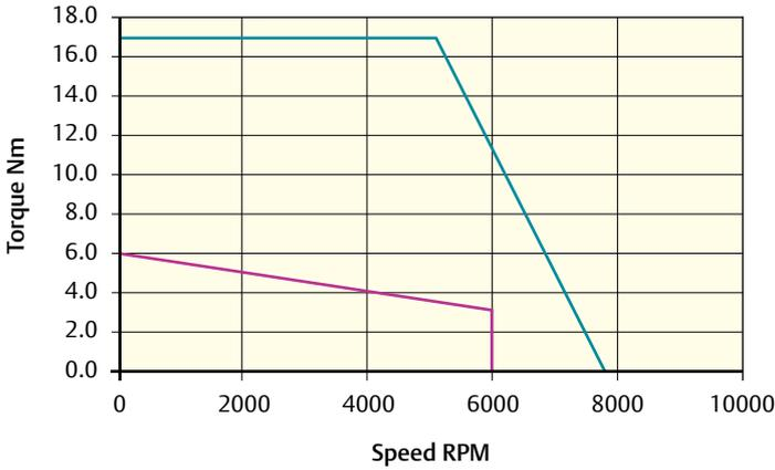
Peak torque (Nm) = 17.1    Stall torque (Nm) = 5.7    Rated torque (Nm) = 2.9
