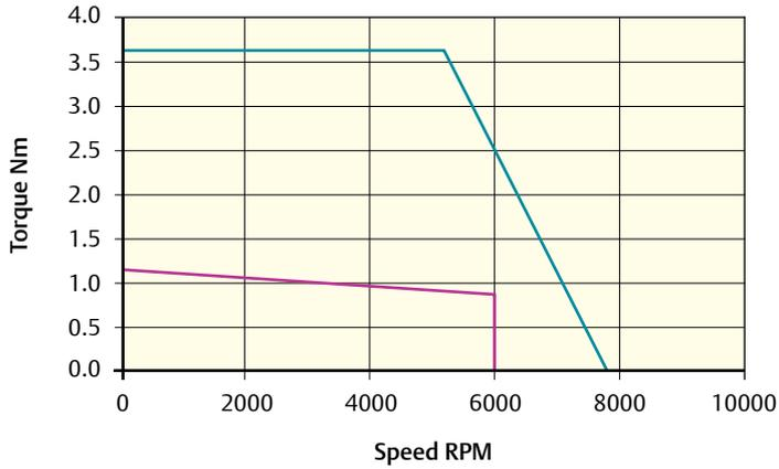
Peak torque (Nm) = 3.6    Stall torque (Nm) = 1.2    Rated torque (Nm) = 0.9
