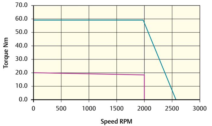
Peak torque (Nm) = 59.4    Stall torque (Nm) = 19.8    Rated torque (Nm) = 18.4
