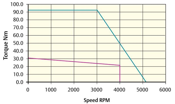
Peak torque (Nm) = 93.3    Stall torque (Nm) = 31.1    Rated torque (Nm) = 21.5
