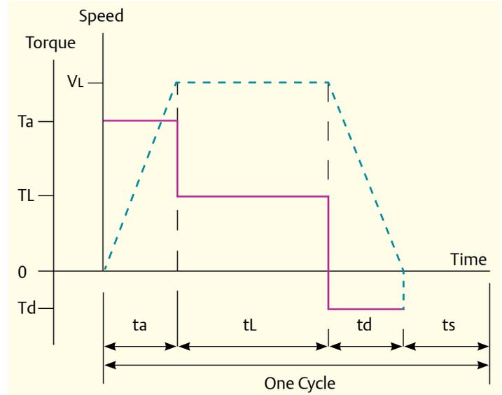
From the above speed-torque diagram calculate the rms torque using the formula:
