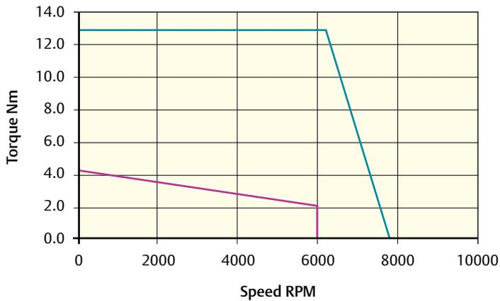
Peak torque (Nm) = 12.9    Stall torque (Nm) = 4.3    Rated torque (Nm) = 2.1
