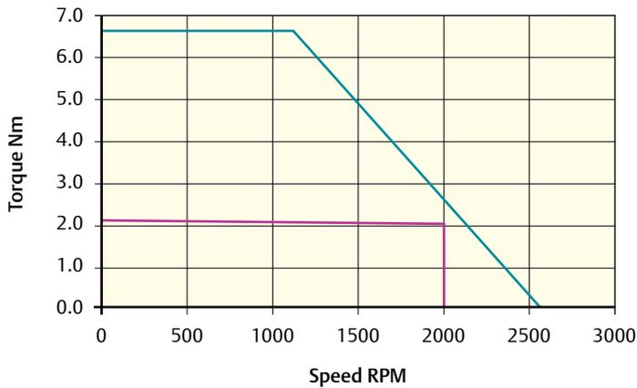
Peak torque (Nm) = 6.6    Stall torque (Nm) = 2.2    Rated torque (Nm) = 2.1
