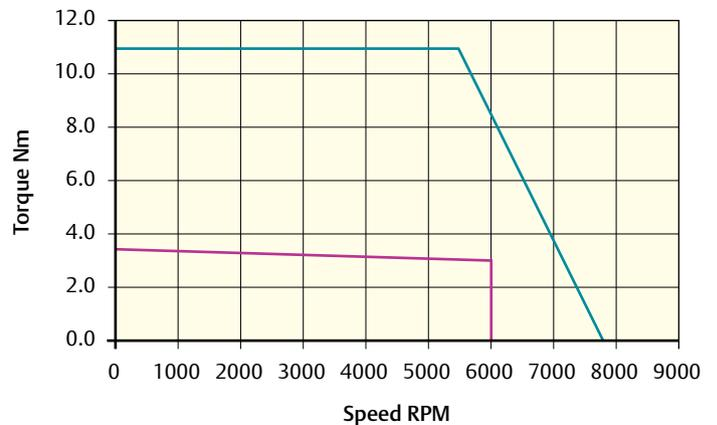
Peak torque (Nm) = 11.10    Stall torque (Nm) = 3.70    Rated torque (Nm) = 3.10
