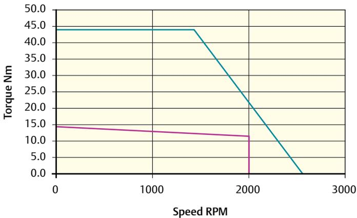
Peak torque (Nm) = 43.80 Stall torque (Nm) = 14.60 Rated torque (Nm) = 11.90
