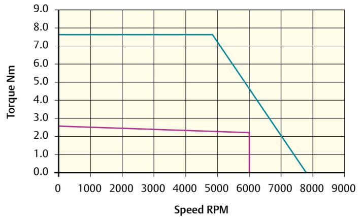
Peak torque (Nm) = 7.65    Stall torque (Nm) = 2.55    Rated torque (Nm) = 2.20
