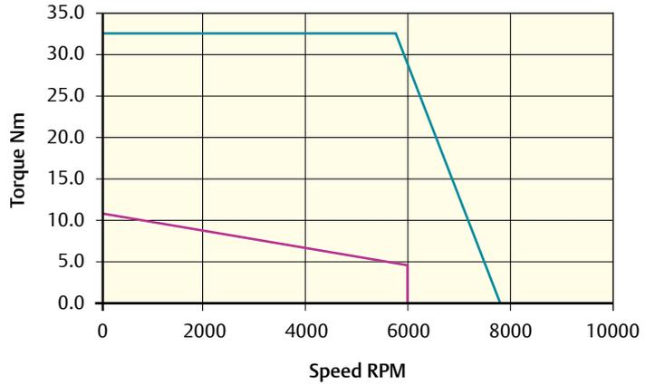
Peak torque (Nm) = 32.4    Stall torque (Nm) = 10.8    Rated torque (Nm) = 4.5
