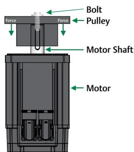
Screw the bolt into the tapped hole of the shaft and, while holding the pulley, use it to push the pulley down and pull the shaft through at the same time.
