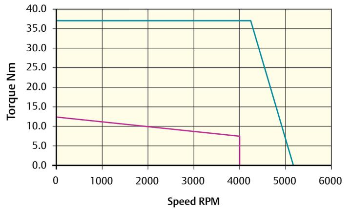
Peak torque (Nm) = 37.2    Stall torque (Nm) = 12.4    Rated torque (Nm) = 7.5
