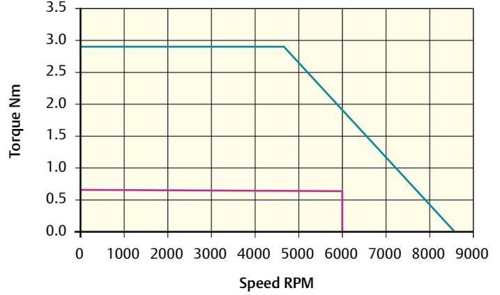
Peak torque (Nm) = 2.88    Stall torque (Nm) = 0.72    Rated torque (Nm) = 0.68
