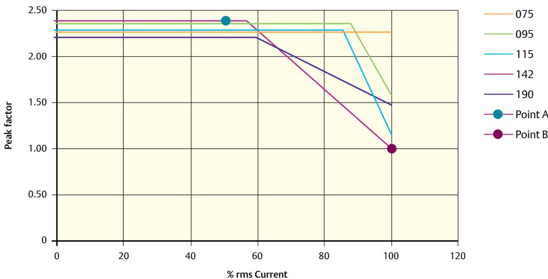
Peak torque is defined for a maximum period of 250ms, rms 3000rpm,  $\Delta_{max} = 100^{\circ}\text{C}$ ,  $40^{\circ}\text{C}$  ambient
