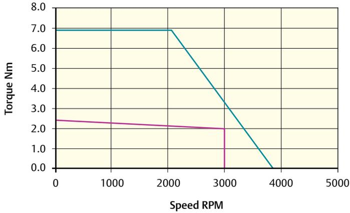
Peak torque (Nm) = 6.9    Stall torque (Nm) = 2.3    Rated torque (Nm) = 2.0
