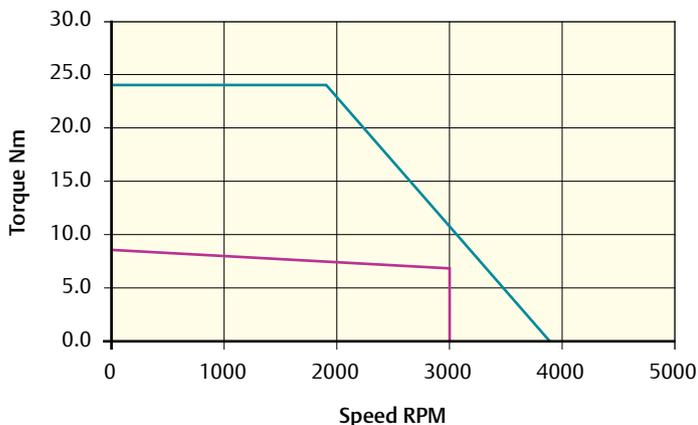
Peak torque (Nm) = 24.00 Stall torque (Nm) = 8.00 Rated torque (Nm) = 6.90
