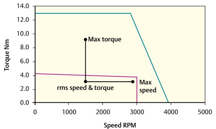
Max torque = 10Nm: Max speed = 2900 rms torque = 3Nm: rms speed = 1500
