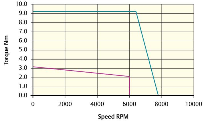
Peak torque (Nm) = 9.3    Stall torque (Nm) = 3.1    Rated torque (Nm) = 2.1
