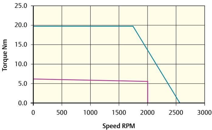
Peak torque (Nm) = 19.8    Stall torque (Nm) = 6.6    Rated torque (Nm) = 6.1
