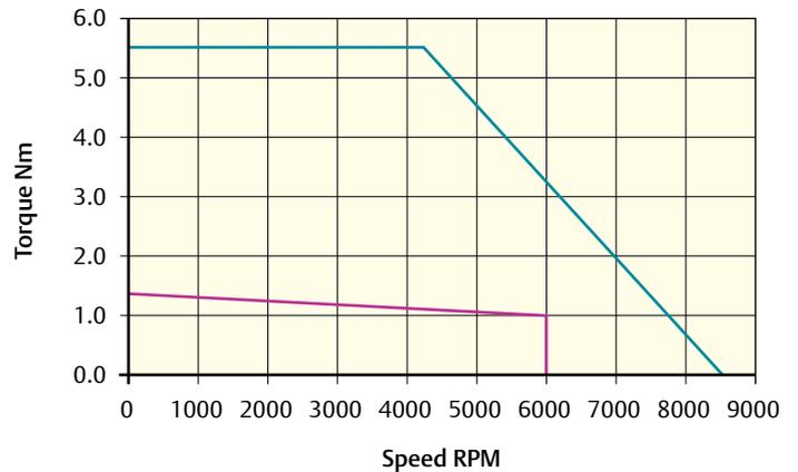
Peak torque (Nm) = 5.5    Stall torque (Nm) = 1.4    Rated torque (Nm) = 0.9
