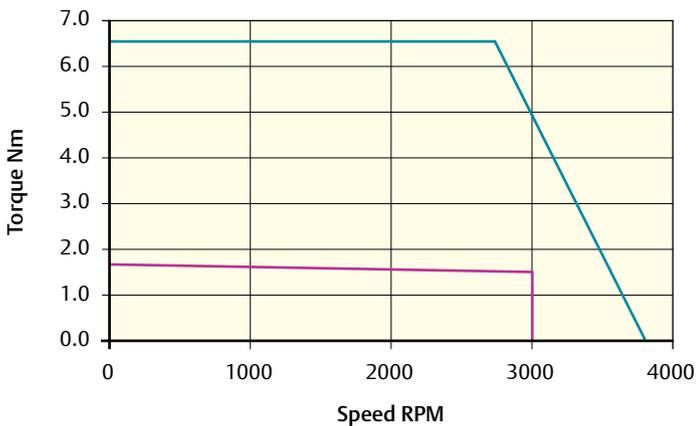
Peak torque (Nm) = 6.60    Stall torque (Nm) = 1.65    Rated torque (Nm) = 1.48
