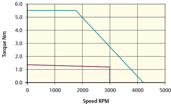
Peak torque (Nm) = 5.5    Stall torque (Nm) = 1.4    Rated torque (Nm) = 1.2
