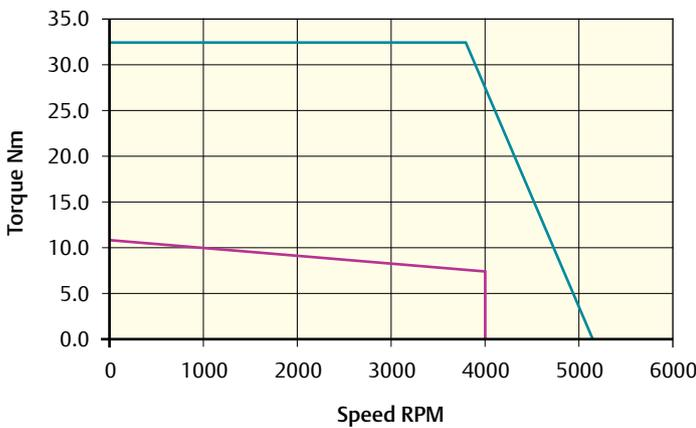
Peak torque (Nm) = 32.4    Stall torque (Nm) = 10.8    Rated torque (Nm) = 7.0
