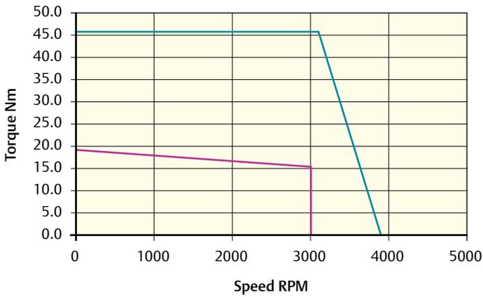
Peak torque (Nm) = 45.90 Stall torque (Nm) = 18.90 Rated torque (Nm) = 16.1
