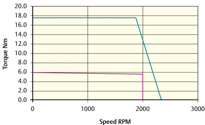
Peak torque (Nm) = 17.7    Stall torque (Nm) = 5.9    Rated torque (Nm) = 5.5
