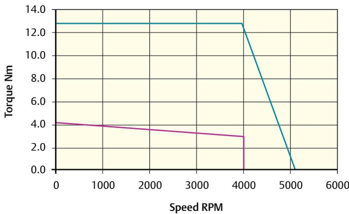
Peak torque (Nm) = 12.9    Stall torque (Nm) = 4.3    Rated torque (Nm) = 3.0
