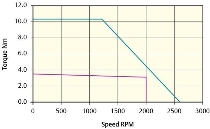
Peak torque (Nm) = 10.5    Stall torque (Nm) = 3.5    Rated torque (Nm) = 3.2
