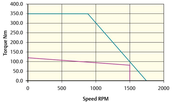
Peak torque (Nm) = 348.0 Stall torque (Nm) = 116.0 Rated torque (Nm) = 76.0
