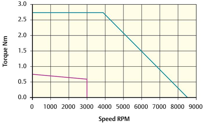
Peak torque (Nm) = 2.8    Stall torque (Nm) = 0.7    Rated torque (Nm) = 0.6
