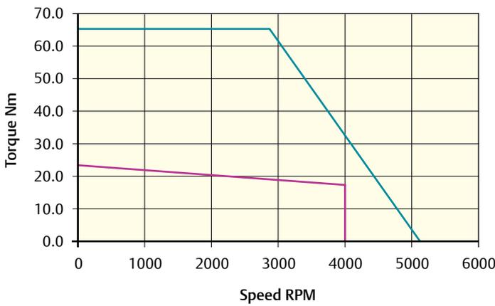
Peak torque (Nm) = 65.4    Stall torque (Nm) = 21.8    Rated torque (Nm) = 17.5
