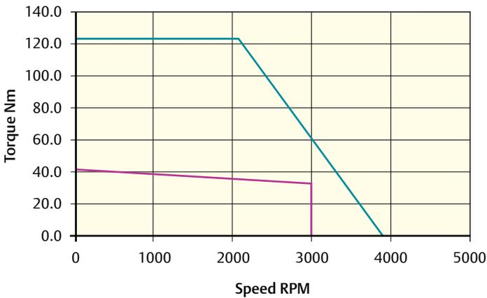
Peak torque (Nm) = 123.3 Stall torque (Nm) = 41.1 Rated torque (Nm) = 33.0
