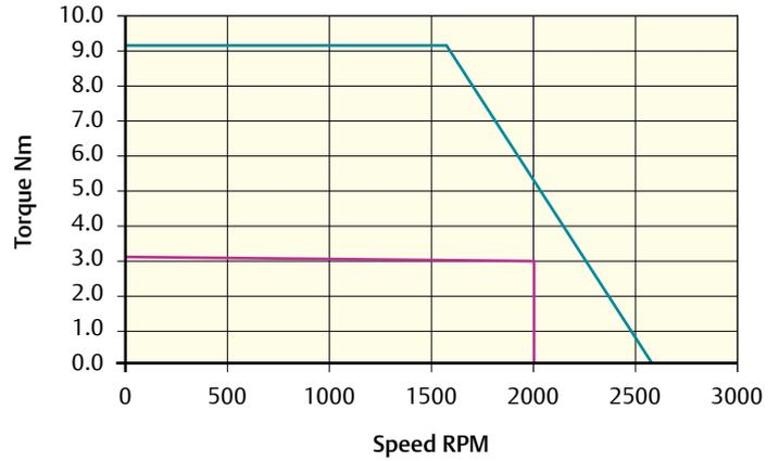
Peak torque (Nm) = 9.3    Stall torque (Nm) = 3.1    Rated torque (Nm) = 3.0
