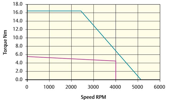
Peak torque (Nm) = 16.50 Stall torque (Nm) = 5.50 Rated torque (Nm) = 4.55
