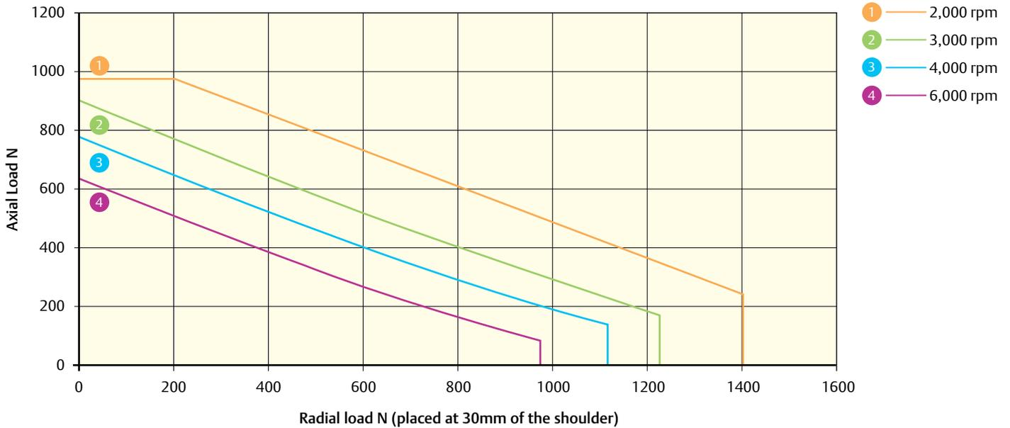
142U2  $L_{10(h)}$  Bearing life for 20,000 hours (reliability 90%, load factor of 1). Do not exceed a maximum axial load of 950 N
