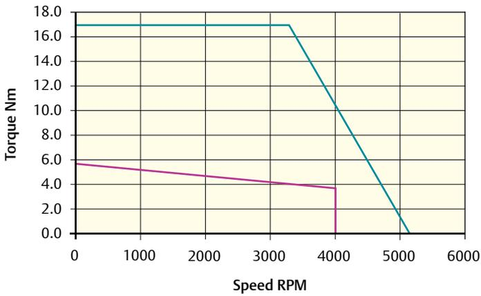
Peak torque (Nm) = 17.1    Stall torque (Nm) = 5.7    Rated torque (Nm) = 3.6
