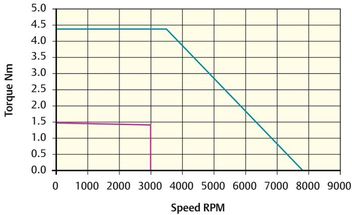
Peak torque (Nm) = 4.35    Stall torque (Nm) = 1.45    Rated torque (Nm) = 1.40
