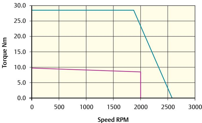
Peak torque (Nm) = 28.2    Stall torque (Nm) = 9.4    Rated torque (Nm) = 8.7
