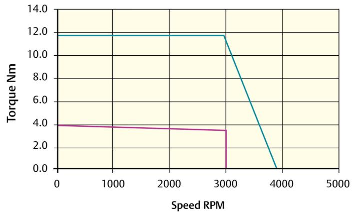
Peak torque (Nm) = 11.7    Stall torque (Nm) = 3.9    Rated torque (Nm) = 3.5
