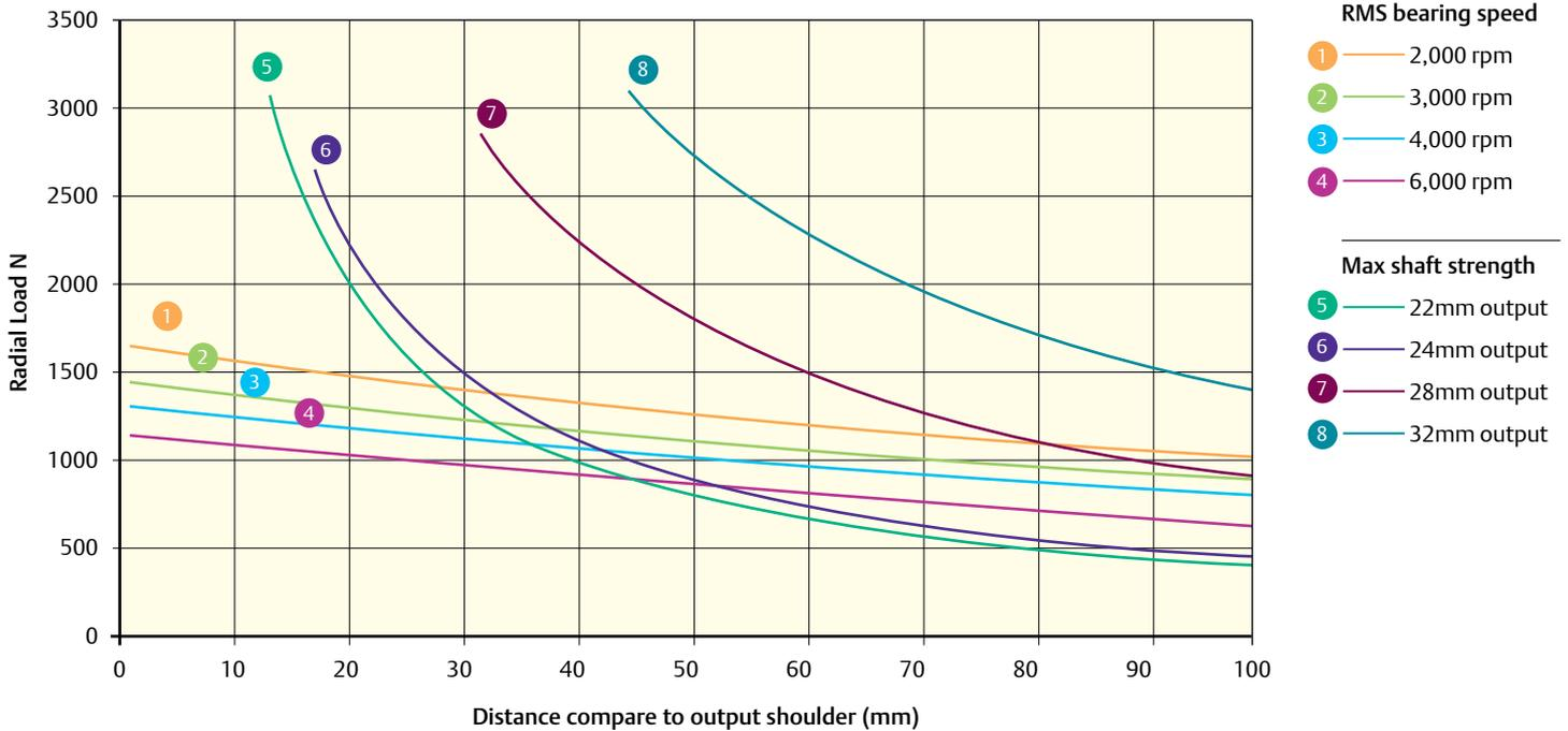
142U2 L<sub>10(h)</sub> Bearing life for 20,000 hours (reliability 90%, load factor of 1)
