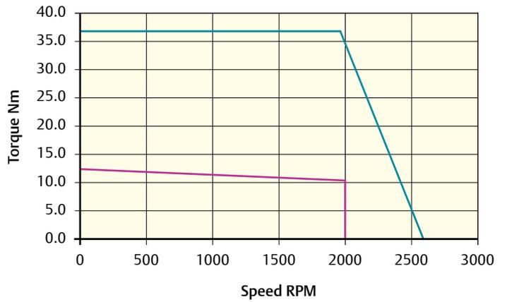
Peak torque (Nm) = 37.2    Stall torque (Nm) = 12.4    Rated torque (Nm) = 10.8
