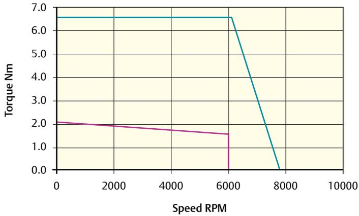
Peak torque (Nm) = 6.6    Stall torque (Nm) = 2.2    Rated torque (Nm) = 1.6
