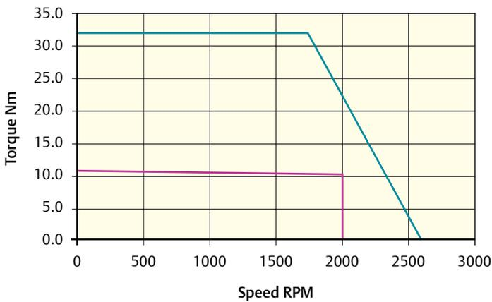
Peak torque (Nm) = 32.4    Stall torque (Nm) = 10.8    Rated torque (Nm) = 10.3
