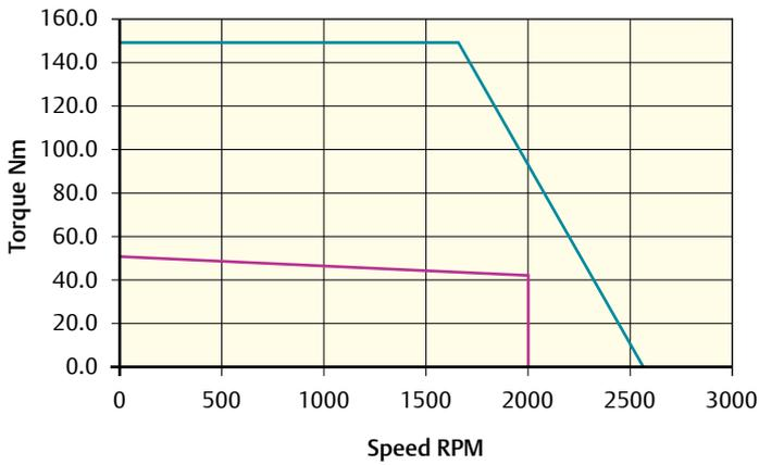
Peak torque (Nm) = 151.6   Stall torque (Nm) = 50.6   Rated torque (Nm) = 43.8
