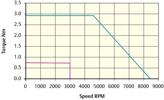
Peak torque (Nm) = 2.88    Stall torque (Nm) = 0.72    Rated torque (Nm) = 0.70
