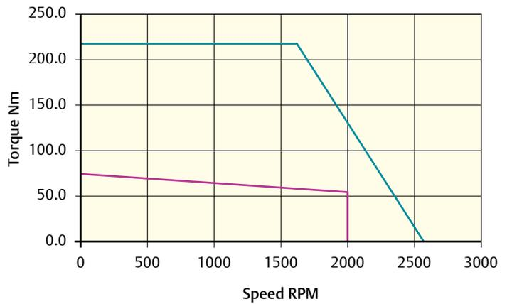
Peak torque (Nm) = 219.6   Stall torque (Nm) = 73.2   Rated torque (Nm) = 54.7
