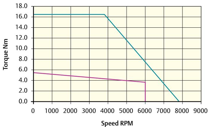
Peak torque (Nm) = 16.50    Stall torque (Nm) = 5.50    Rated torque (Nm) = 3.80
