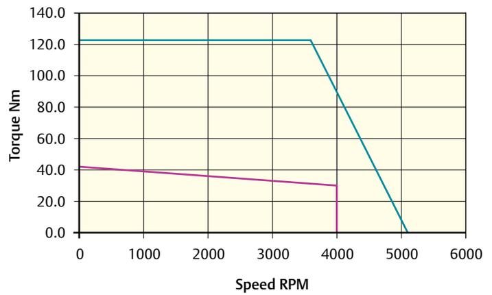
Peak torque (Nm) = 123.3    Stall torque (Nm) = 41.1    Rated torque (Nm) = 29.0
