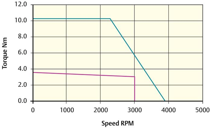
Peak torque (Nm) = 10.5    Stall torque (Nm) = 3.5    Rated torque (Nm) = 3.0
