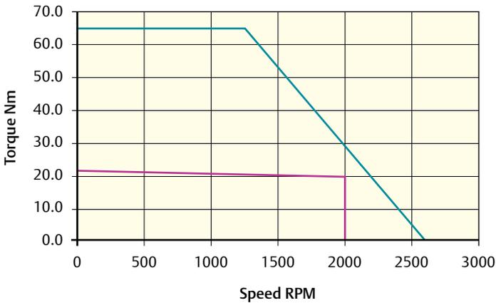
Peak torque (Nm) = 65.4    Stall torque (Nm) = 21.8    Rated torque (Nm) = 20.0
