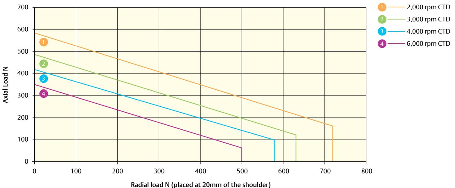
75U2 L<sub>10(h)</sub> Bearing life for 20,000 hours (reliability 90%, load factor of 1). Do not exceed a maximum axial load of 900 N
