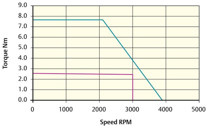
Peak torque (Nm) = 7.65    Stall torque (Nm) = 2.55    Rated torque (Nm) = 2.45
