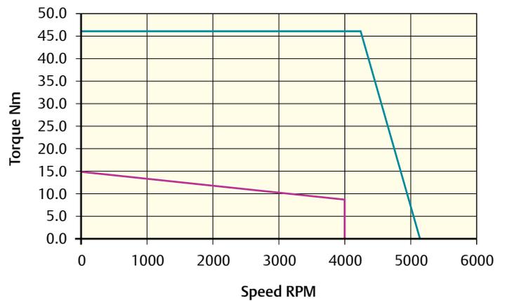
Peak torque (Nm) = 45.9    Stall torque (Nm) = 15.3    Rated torque (Nm) = 8.7
