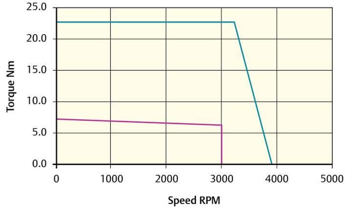
Peak torque (Nm) = 22.5    Stall torque (Nm) = 7.5    Rated torque (Nm) = 6.8
