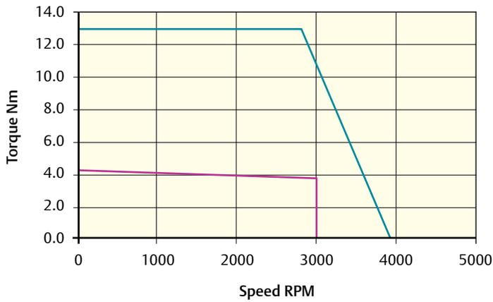
Peak torque (Nm) = 12.9    Stall torque (Nm) = 4.3    Rated torque (Nm) = 3.9
