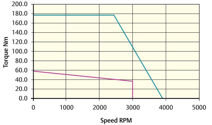
Peak torque (Nm) = 176.1 Stall torque (Nm) = 58.7 Rated torque (Nm) = 35.0
