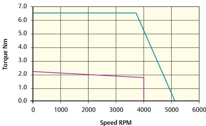
Peak torque (Nm) = 6.6    Stall torque (Nm) = 2.2    Rated torque (Nm) = 1.7
