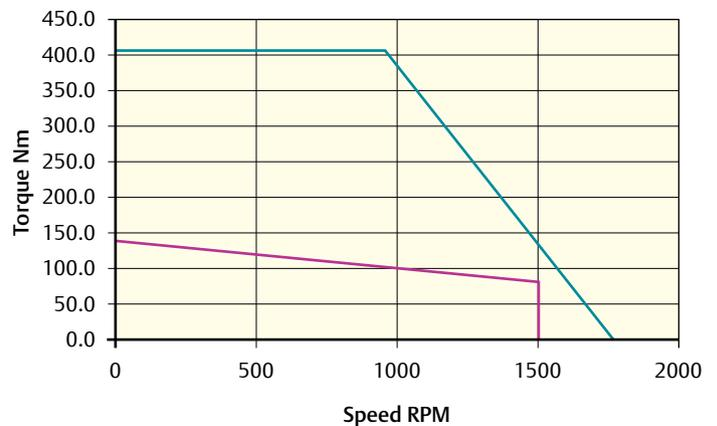
Peak torque (Nm) = 408.0 Stall torque (Nm) = 136.0 Rated torque (Nm) = 84.0
