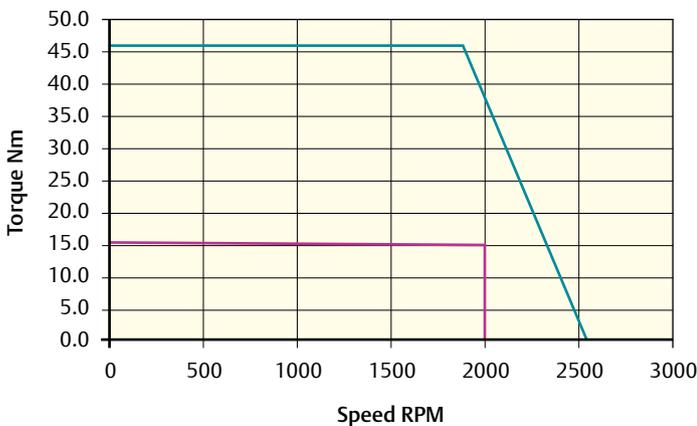
Peak torque (Nm) = 45.9    Stall torque (Nm) = 15.3    Rated torque (Nm) = 14.6
