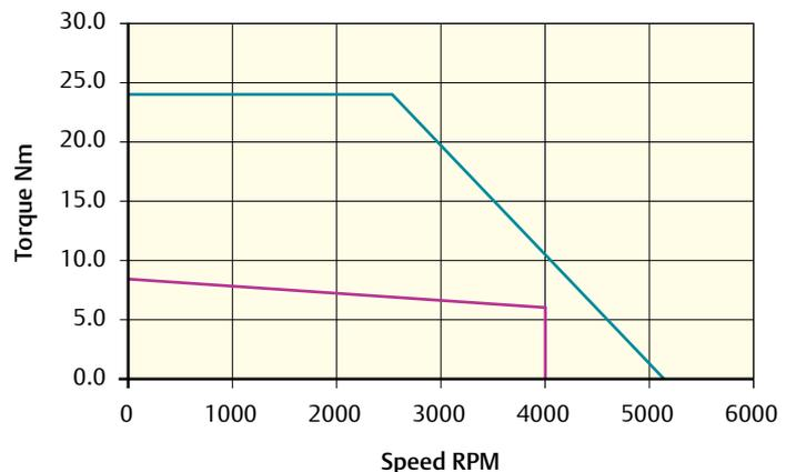
Peak torque (Nm) = 24.00 Stall torque (Nm) = 8.00 Rated torque (Nm) = 6.35
