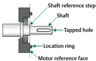
The diagram left shows the front face of the Unimotor, when using the following instructions the component hub should be drawn against the shaft reference step, which is in line with the motor reference face.
