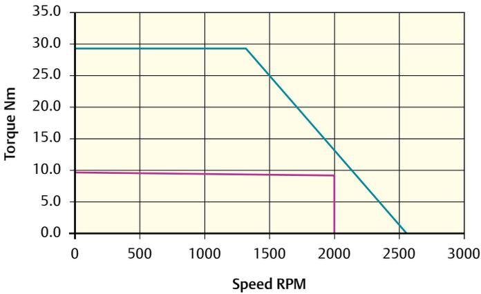
Peak torque (Nm) = 28.2    Stall torque (Nm) = 9.6    Rated torque (Nm) = 9.3
