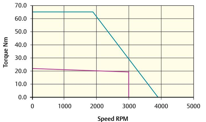
Peak torque (Nm) = 65.4   Stall torque (Nm) = 21.8   Rated torque (Nm) = 19.5
