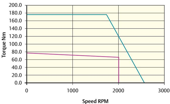
Peak torque (Nm) = 176.10 Stall torque (Nm) = 79.0 Rated torque (Nm) = 66.5
