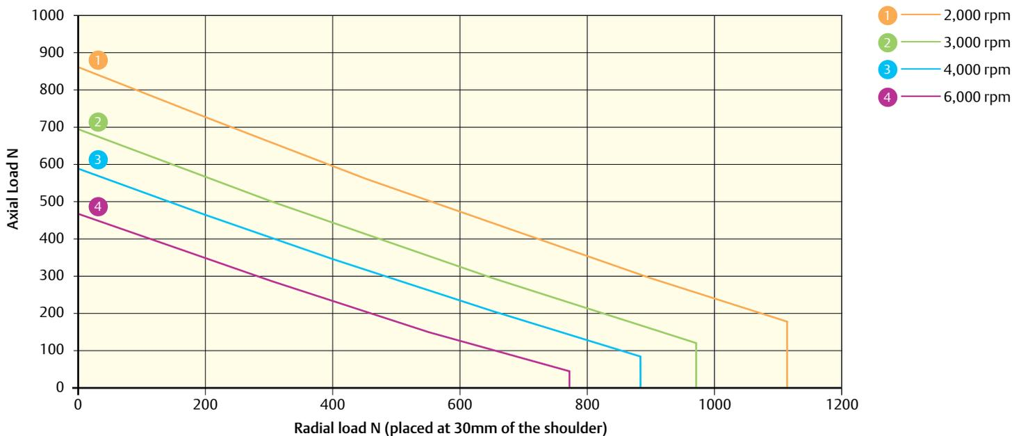
115UD  $L_{10(h)}$  Bearing life for 20,000 hours (reliability 90%, load factor of 1). Do not exceed a maximum axial load of 1200 N
