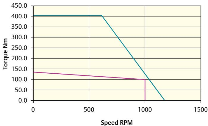
Peak torque (Nm) = 408.0 Stall torque (Nm) = 136.0 Rated torque (Nm) = 106.0
