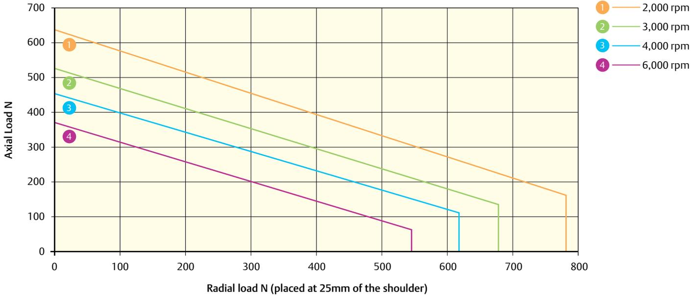
95U2  $L_{10(h)}$  Bearing life for 20,000 hours (reliability 90%, load factor of 1). Do not exceed a maximum axial load of 850 N
