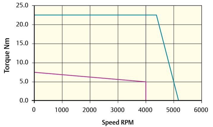
Peak torque (Nm) = 22.5    Stall torque (Nm) = 7.5    Rated torque (Nm) = 4.9
