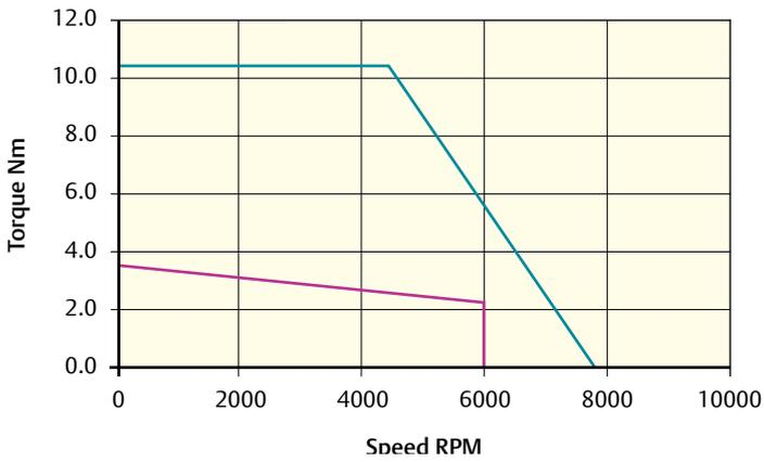
Peak torque (Nm) = 10.5    Stall torque (Nm) = 3.5    Rated torque (Nm) = 2.2
