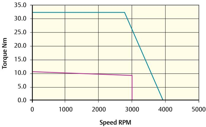
Peak torque (Nm) = 32.4    Stall torque (Nm) = 10.8    Rated torque (Nm) = 9.0
