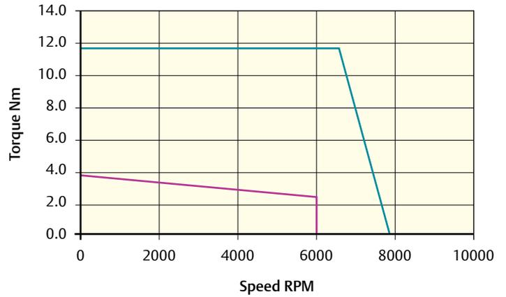
Peak torque (Nm) = 11.7    Stall torque (Nm) = 3.9    Rated torque (Nm) = 2.6
