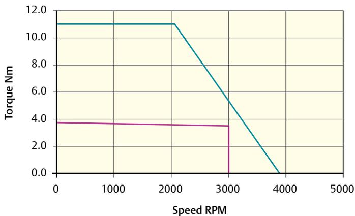
Peak torque (Nm) = 11.10    Stall torque (Nm) = 3.70    Rated torque (Nm) = 3.50
