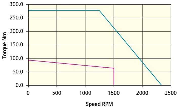
Peak torque (Nm) = 276.0 Stall torque (Nm) = 92.0 Rated torque (Nm) = 65.0
