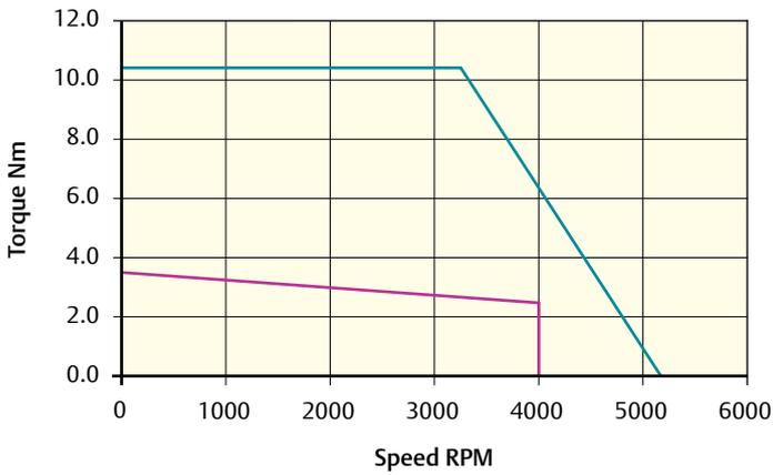
Peak torque (Nm) = 10.5    Stall torque (Nm) = 3.5    Rated torque (Nm) = 2.5
