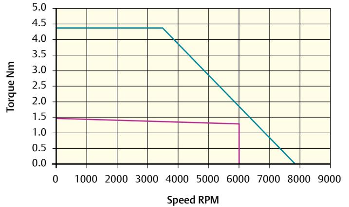
Peak torque (Nm) = 4.35    Stall torque (Nm) = 1.45    Rated torque (Nm) = 1.30
