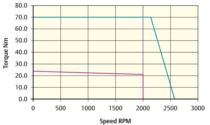
Peak torque (Nm) = 70.4    Stall torque (Nm) = 23.4    Rated torque (Nm) = 21.3
