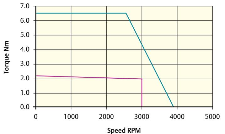
Peak torque (Nm) = 6.6    Stall torque (Nm) = 2.2    Rated torque (Nm) = 2.0
