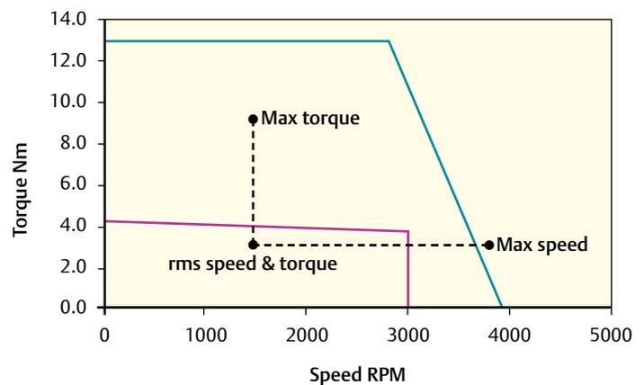
Max torque = 10Nm: Max speed = 3900 rms torque = 3Nm: rms speed = 1500
