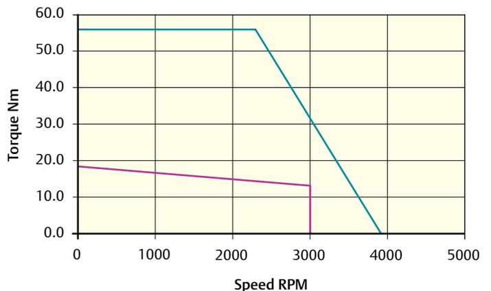
Peak torque (Nm) = 56.40 Stall torque (Nm) = 18.80 Rated torque (Nm) = 13.60
