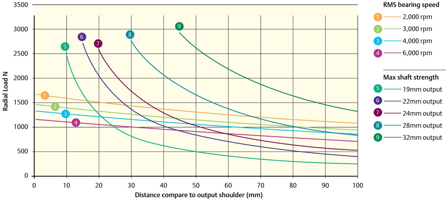
115U2 L<sub>10(h)</sub> Bearing life for 20,000 hours (reliability 90%, load factor of 1)
