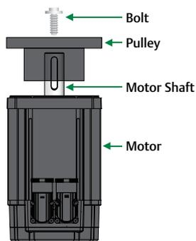
When fitting a pulley, a system that pushes the pulley down the shaft while pulling the shaft up through the pulley should be applied. A simple technique is to use a bolt with a washer.
