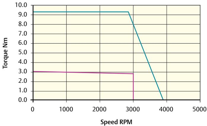
Peak torque (Nm) = 9.3    Stall torque (Nm) = 3.1    Rated torque (Nm) = 2.8
