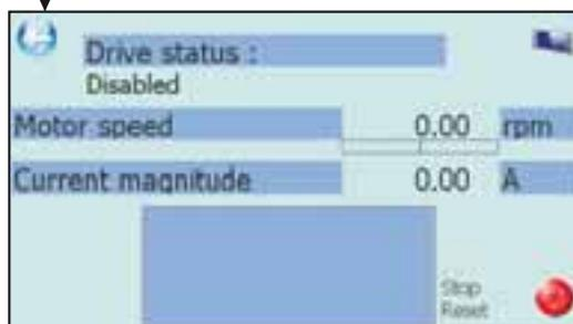
By default, the screen gives Informations about the drive status, the calculated motor speed and the current magnitude. The Stop/Reset command is also active.
