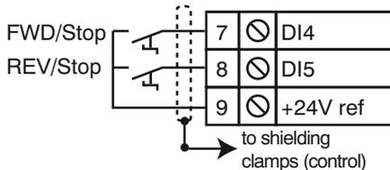
On power-up or after a trip reset, if a run command is already selected, the motor does not start. The Run input (DI4 or DI5) must be cycled for the command to take effect.
