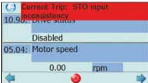
To clear a trip: resolve the problem, then press the Stop/Reset button. If necessary, see section 7 - Trips - Diagnostics.
