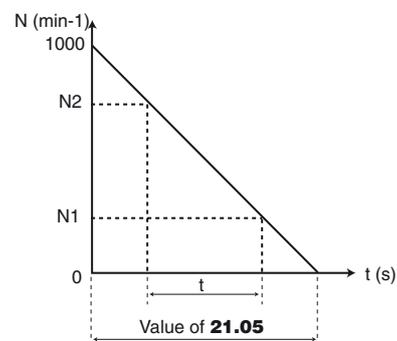
This parameter is equivalent to **02.21** in motor 1.
