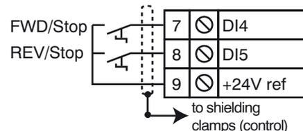
On power-up or after a trip reset, if a Run command is already selected, the motor starts as soon as the speed reference appears.
