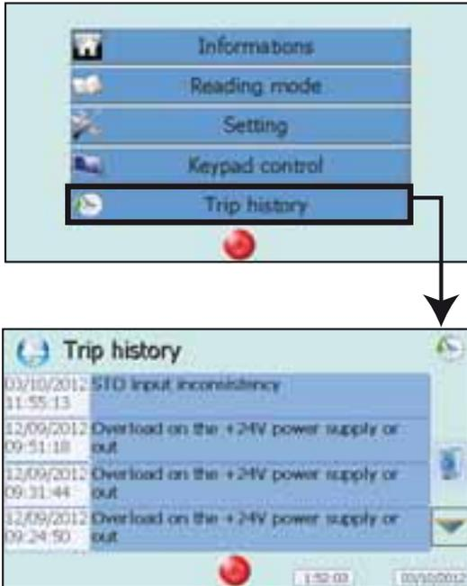
When the drive trips, it is displayed in a red banner, at the top of the interface screen. When the drive trips an alarm, it is displayed in an orange banner.
