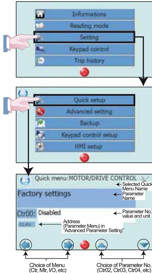
For a more detailed explanation of the menus and parameters offered in "Quick setup", refer to section 4.
