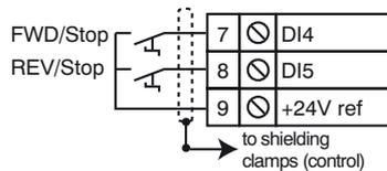
On power-up or after a trip reset, if a Run command is already selected, the motor starts as soon as the speed reference appears.
