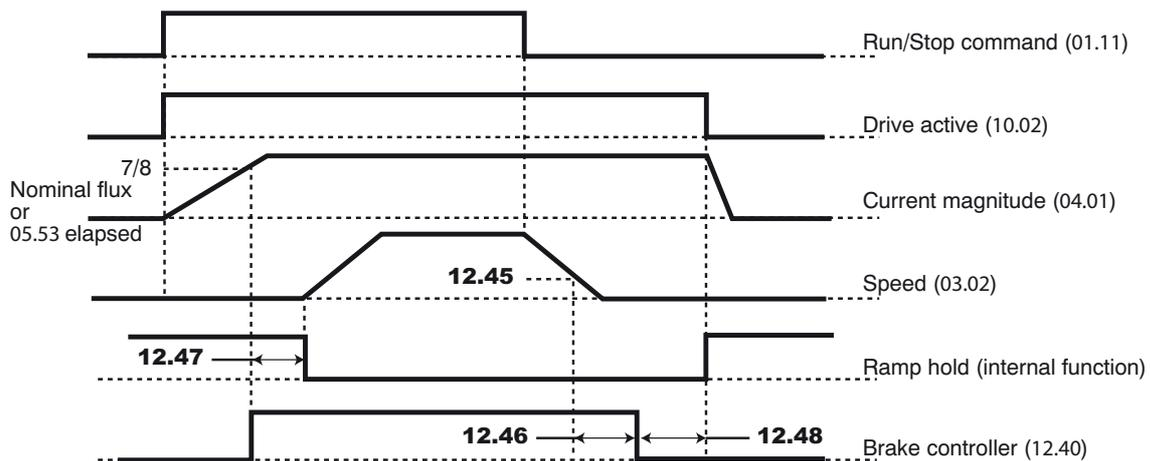
**POWERDRIVE MD2/FX****Variable speed drive****ADVANCED PARAMETER-SETTING MODE****5.13.2 - Explanation of parameters in menu 12****12.01** : Comparator 1 output**12.02** : Comparator 2 output
