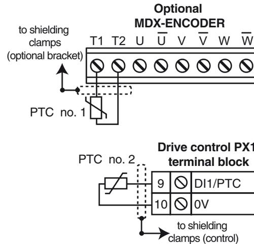
**CAUTION:** If **Mtr.06** is set to "Drive terminal" or "2 PTC inputs", then digital input DI1 must not be used (do not assign I/O.06).
