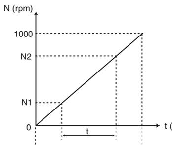
**02.11:** Acceleration rate 1 (main ramp in factory settings)
